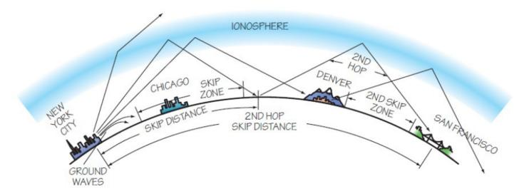
When you transmit a radio wave, it goes toward the ionosphere and skips back to Earth.
